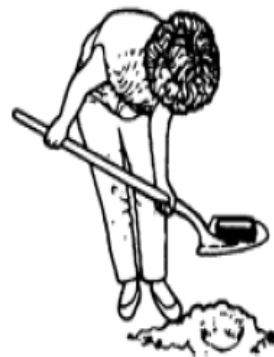
Figure 1b. Use a hand trowel, shovel or other garden tool. Trim out soil of uniform thickness to the recommended depth.
