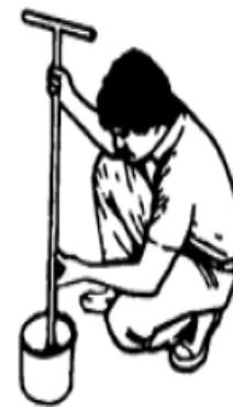
Figure 2. Place 10 to 15 soil cores into a plastic bucket; mix, dry, and transfer to a bag.
